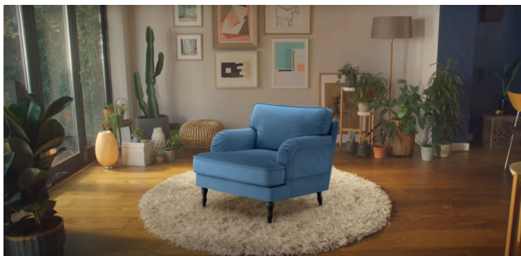
Figure 1.1: A screenshot from the IKEA Places AR application, inserting a virtual couch into the scene. While the results are plausible, the appearance of the couch is noticeably inconsistent with the rest of the scene – the shadow underneath the couch does not match the shadows of the objects on the left side of the image, and the lighting on the couch itself suggests strong overhead lighting, which is not present in the scene itself.
