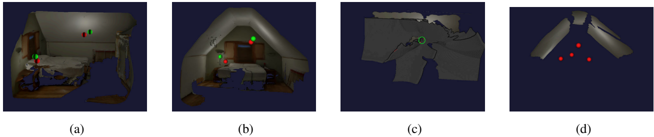
Figure 6.10: Results of running my method on a scanned 3D dataset. 6.10a-6.10b show the scanned scene colored with the averaged observations B(q) . The original light locations are rendered as green spheres, while the recovered light locations are rendered as red spheres. The bottom two images only show the B(q) used in the computation. In 6.10c, the initial medial axis and \mathcal{V}(p) are shown, with a clear maximum (circled in green) at the location of one of the light sources. After a few iterations (6.10d), several more maxima appear (rendered as red spheres); two among these are close enough to the true light positions for the optimization to succeed.
