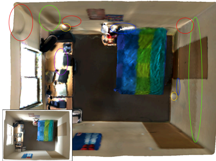
Figure 5.10: I compute a “reflectance mesh” by taking the radiances from the input mesh (inset) and the solved lighting, and compute a per-vertex reflectance as radiance divided by incident light.
