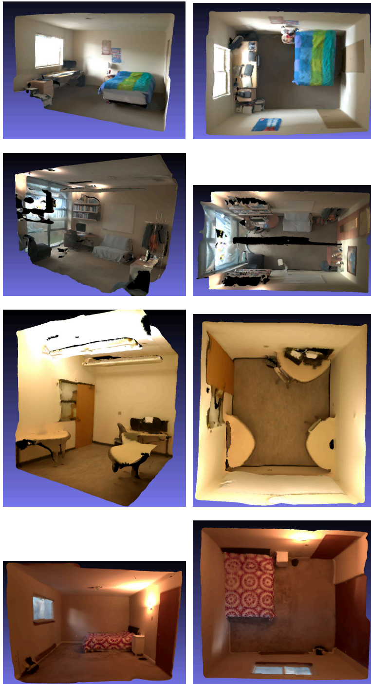
Figure 3.4: Results of the capture system on real scenes. The left column shows a wide angle view of the scene, while the right column shows an overhead view of the scene.
