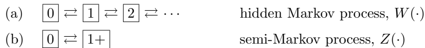
Figure 2.6: State models considered by Crespi et al. (2005). The unobservable number of recurrences at time t is modeled as a birth-death process (a), while the viral shedding status is modeled as the corresponding semi-Markov process (b) defined by collapsing states 1, 2, 3, \dots of the birth-death process.
