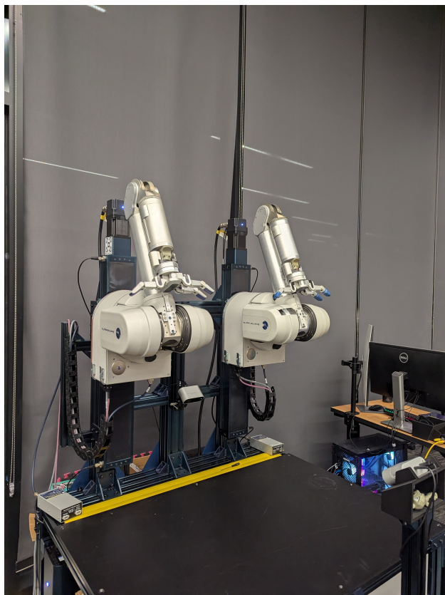
Figure 2.1: The Geodude hardware setup consisting of two 7-DOF Barrett WAM arms, Barrett Hands , stereo cameras and linear actuators
