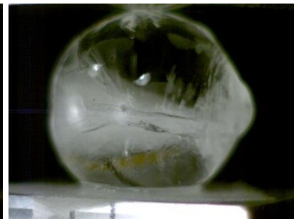
C) Onset of rapid crack propagation t = 0.01116 \text{ sec}
