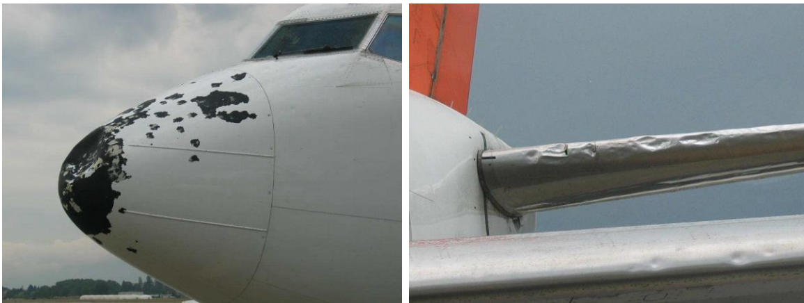
Figure 3: Boeing 737 Hail Strike Damage, 14 Aug 2003 [7]
