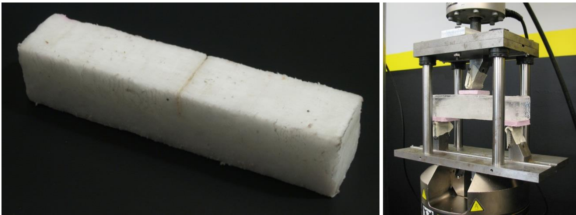
Figure 29: Fracture Toughness Beam Specimen and Test Setup
