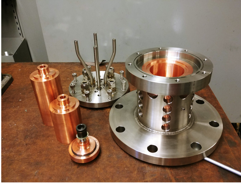
Figure 2.5: Manufactured hardware and swappable engine cores.
