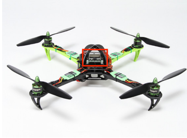
Figure 6.2: Turnigy SK450 quadcopter, with the original flight controller unit highlighted.
