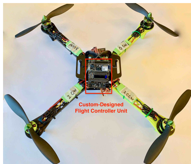
Figure 6.9: A photo of the custom-designed flight controller unit mounted on the quadcopter.
