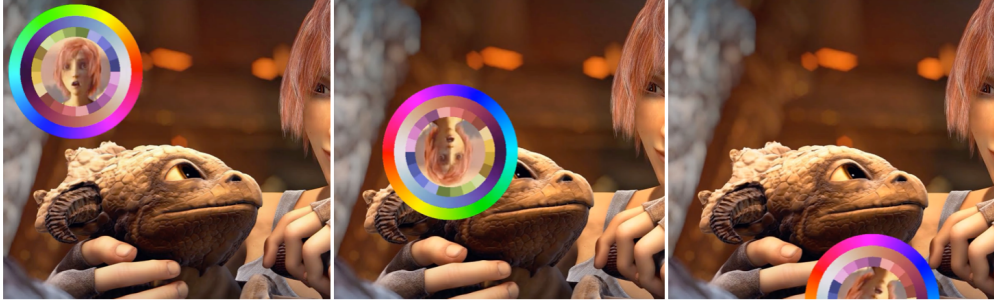
Figure 4.9: Synthetic test sequence. The testing sequence used for evaluating long-term dense motion estimation. The video consists of 600 frames in which a textured disc rotates and bounces around the frame. The background also moves independently from frame-to-frame with a randomly initialized 2D Fourier series, resulting in a frame-to-frame motion of 5-20 pixels per frame.
