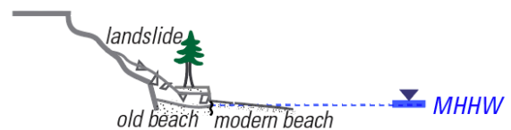
Figure 3.24. Diagram of how an increase in sediment supply can produce observed stratigraphy at Ellen Creek and T1.
