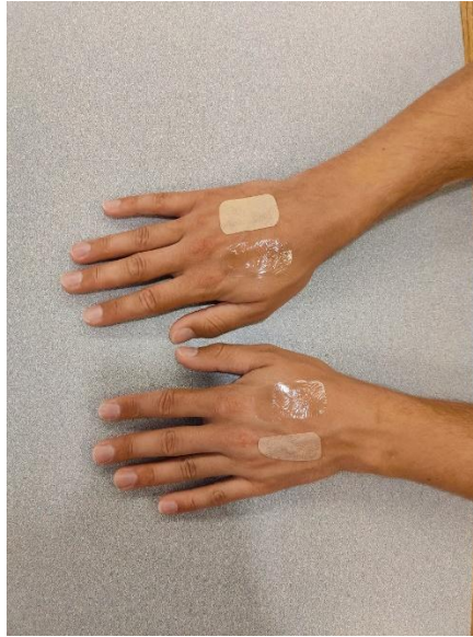
Fig. 4.15: Tapes after application. Sensitive Skin is the darker sample at the bottom of the image, Water Block is the lighter colored sample at the top of the image, and ThermoTape is the two clear transparent tapes.
