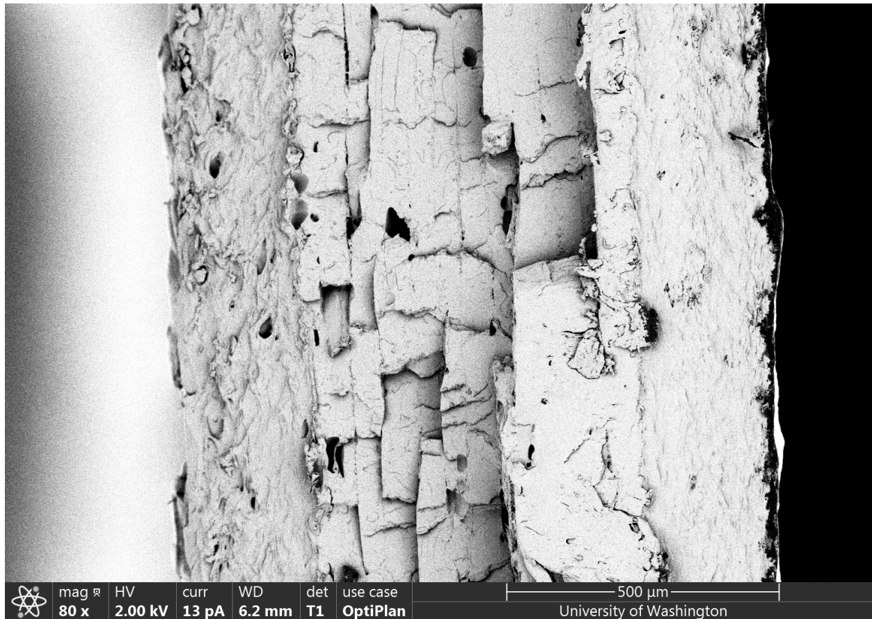
Figure 25: 3D printed 4MPa saturated PLA at extrusion temperature of 180°C
