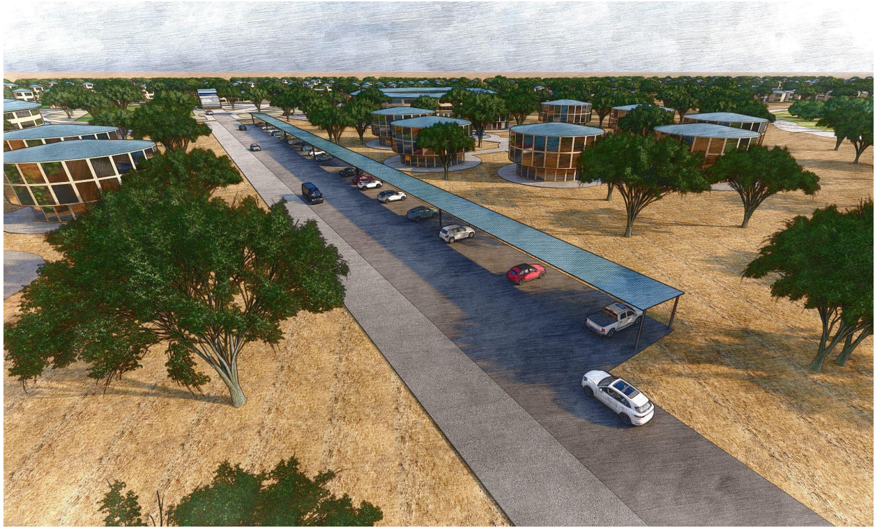
Figure 38. Solar covered carport for AEVs, located along the radial line between a group center and its cluster center.
