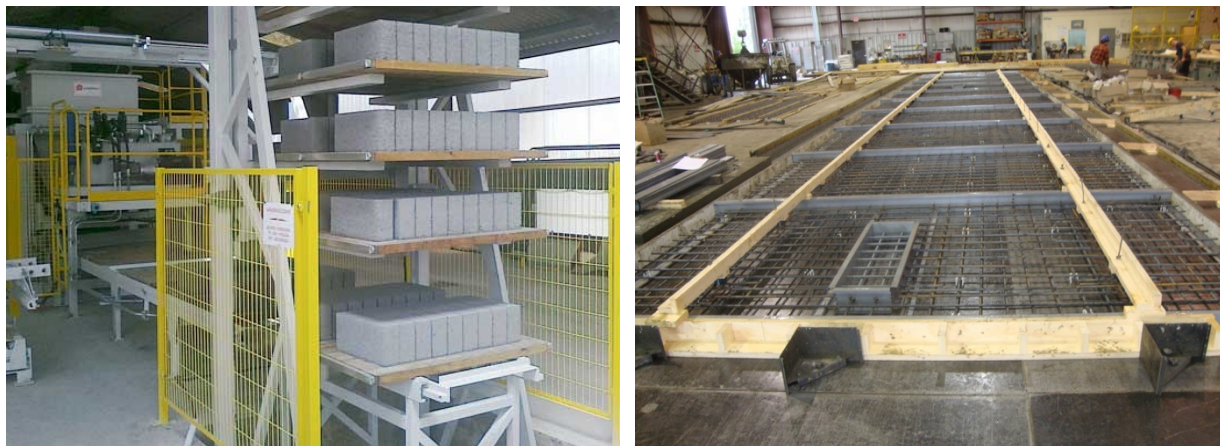
Figure 29. Left: Automated CMU production line. Source: Pyatos. Retrieved from: https://www.poyatos.com/?attachment_id=3715 .
