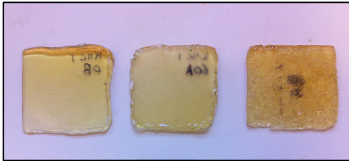
fig. 3: Substrate plates, right to left: smooth, 0.269mm, 1-2mm
