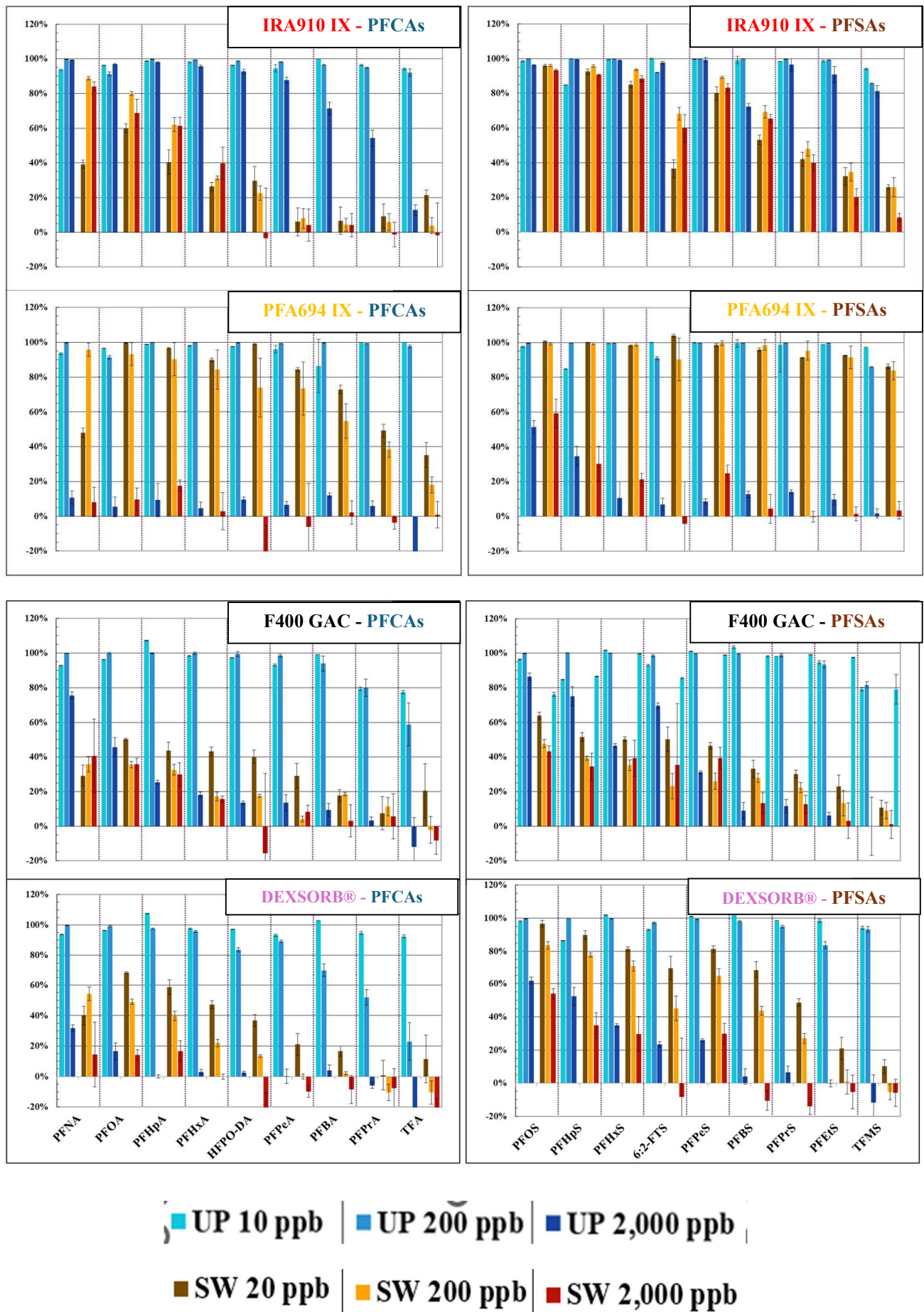
Figure 2.4 compares the results from three of the batch adsorption capacity tests in UP water with nominal initial PFAS concentrations of 10 \mu\text{g/L} , 200 \mu\text{g/L} , and 2 \text{mg/L} (each PFAS) with the three batch adsorption capacity tests conducted in the SW matrix with nominal initial PFAS concentrations of 20 \mu\text{g/L} , 200 \mu\text{g/L} , and 2 \text{mg/L} (each PFAS).
