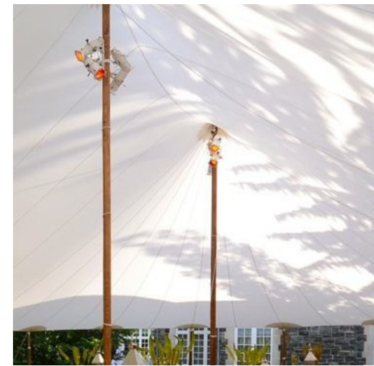
c : coated white polyester (PET) sailcloth over 1''x 1'' hs aluminum frames
