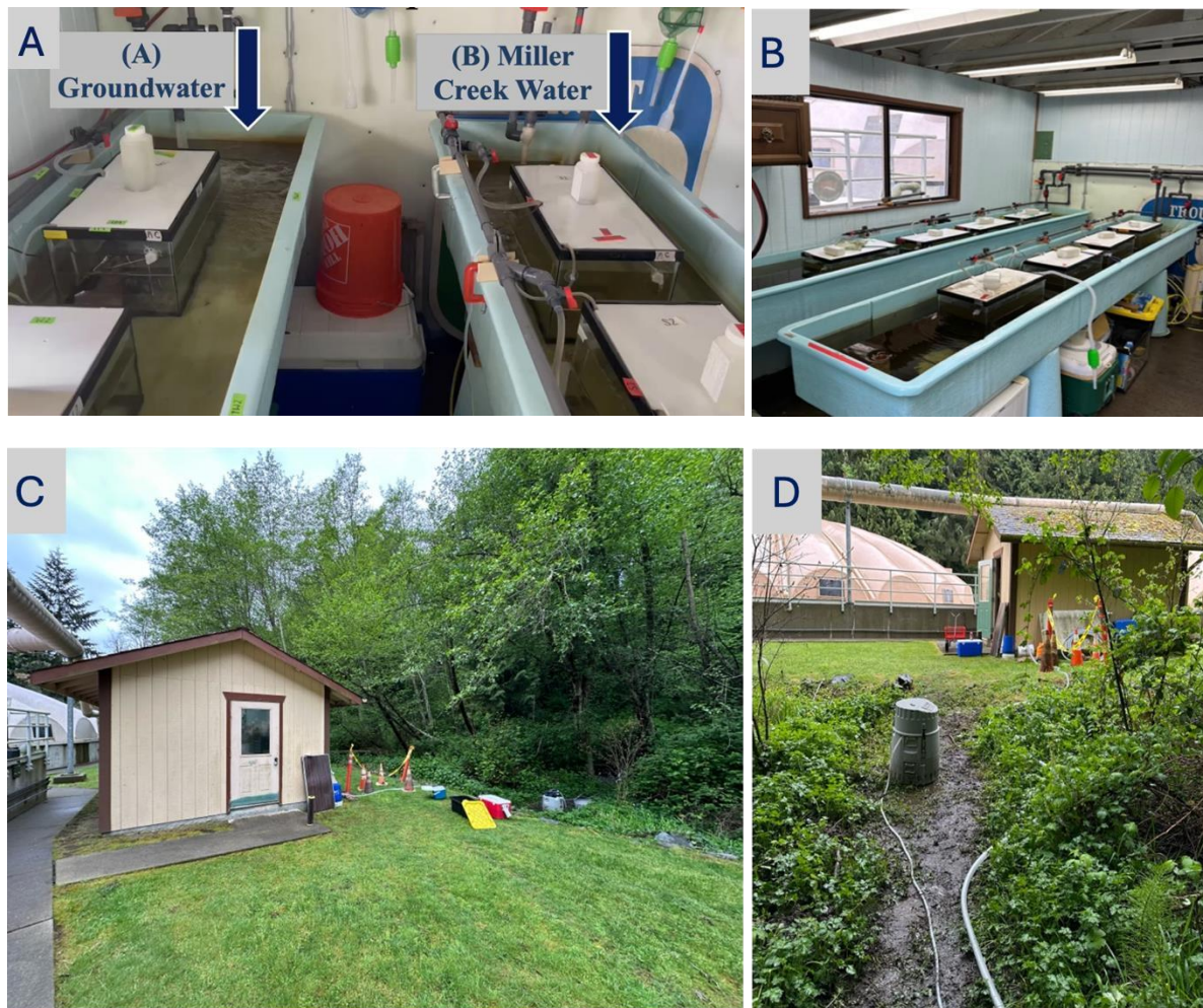
Figure 2.1. Current field Laboratory set up at Miller Creek for real time exposure of targeted storm events. (a) Parallel raceways with flow through groundwater in raceway A and miller creek water in raceway B. (b) Exposure study tank set up including four fish tanks per raceway per storm in each raceway. (c) Image of the field laboratory located along Miller Creek. (d) Image of
