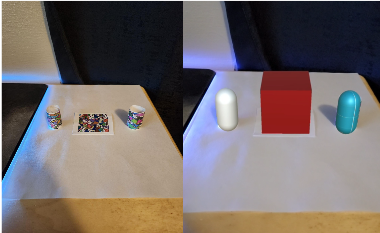
Figure 3.1: Image and cylinder targets (left) and the virtual objects generated by them(right)
