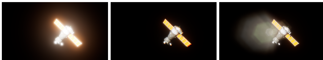
Figure 1.4: Left: Scenarios showing effects of bloom from the surface when camera is suddenly switched on. Middle: Chromatic aberration due to defective lens. Right: Flares due to light scattering
