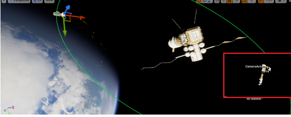
Figure 2.3: Simulation platform showing the Ego (denoted on the left with its attached body frame) orbiting around an uncontrolled satellite Target (the white object in the middle) on a fixed flyby orbit (denoted by a green circle). The in-picture on the right shows the Target in the Ego's camera frame.
