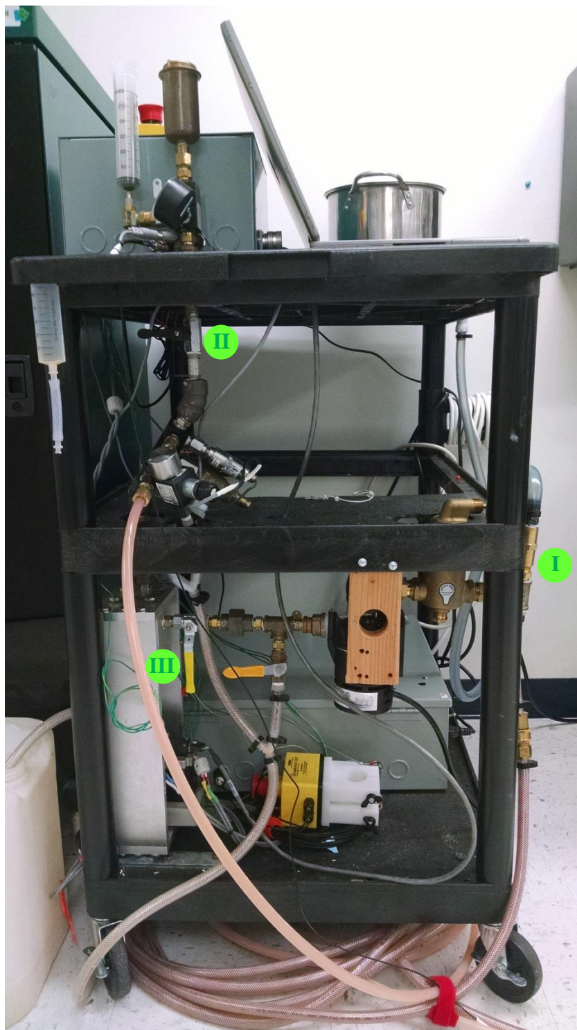
Figure III.1b – Photo of the main HyPSTR cart in the lab. Valves (marked with green circles) I, II, and III should be open when the recirculation pump is on.
