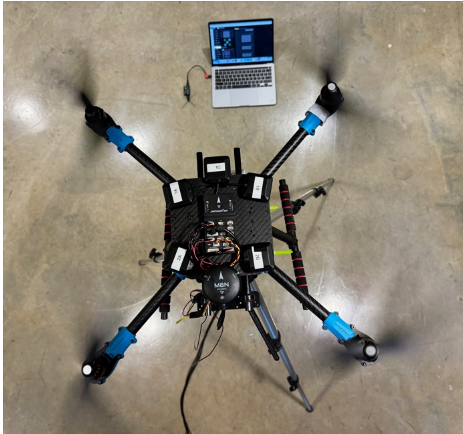
Figure 5-7. UAV Ground Station Integration Test with experimental GPS DAQ Setup on UAV. This image captures a UAV secured to a tripod, with propellers engaged to emulate in-flight dynamics. A wireless transmitter-receiver, visible next to the computer, relays telemetry data in real time, facilitating direct command transmission and live data monitoring to replicate true flight conditions for rigorous system validation. The antennas of the test system, marked with white labels, are positioned on the drone's extremities to ensure wide sky visibility and accurate signal reception. At the rear, above the propellers for a M8N GPS antenna compatible with the drone's flight controller is mounted.
