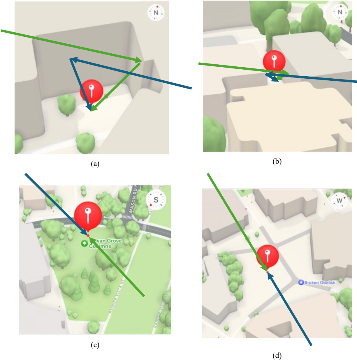
Figure 7-16. Isometric 3D view of GPS test locations illustrating signal reflection challenges. The green arrow represents the signal from a satellite at first acquisition, and purple the last signal received from the satellite before line sight is lost. (a) Urban location 1 with a narrow alley enclosed by high walls, illustrating substantial GPS signal reflection and multipath effects due to the urban canyon environment. (b) Urban location 3 is bordered by tall buildings on two sides, with a third reflector in the southerly direction a distance away. It depicts a lower level of GPS signal interference with more open sky visibility compared to urban location 1. (c) Urban location 2 with ‘soft’ obstacles (vegetation with varying density) and marble columns to the north, showing mixed GPS signal reception conditions due to partial blockage on one side. (d) Semi-urban, a relatively more open area with obstructions for GPS signals located near the test field's edge with clear line-of-sight access to the sky in the center of the reception field, indicative of more favorable conditions for GPS reception.
