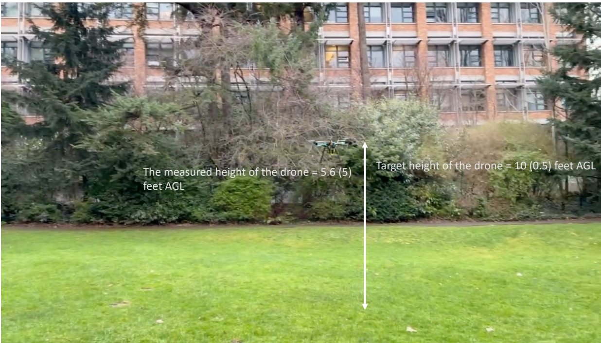
Figure 4-3. Altitude Discrepancy During Corridor Scan Test. Captured at the University of Washington, this still shows the drone's actual flight altitude at 5.6 feet AGL, contrasting with the targeted 10 feet AGL. Such deviation may stem from localization errors, suboptimal GPS signal quality, or barometric pressure variations affecting sensor accuracy.
