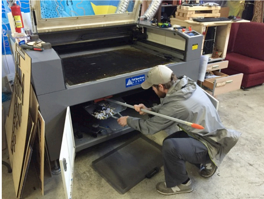
Figure 8. Eric cleans debris from previous cuts on the laser cutter.
