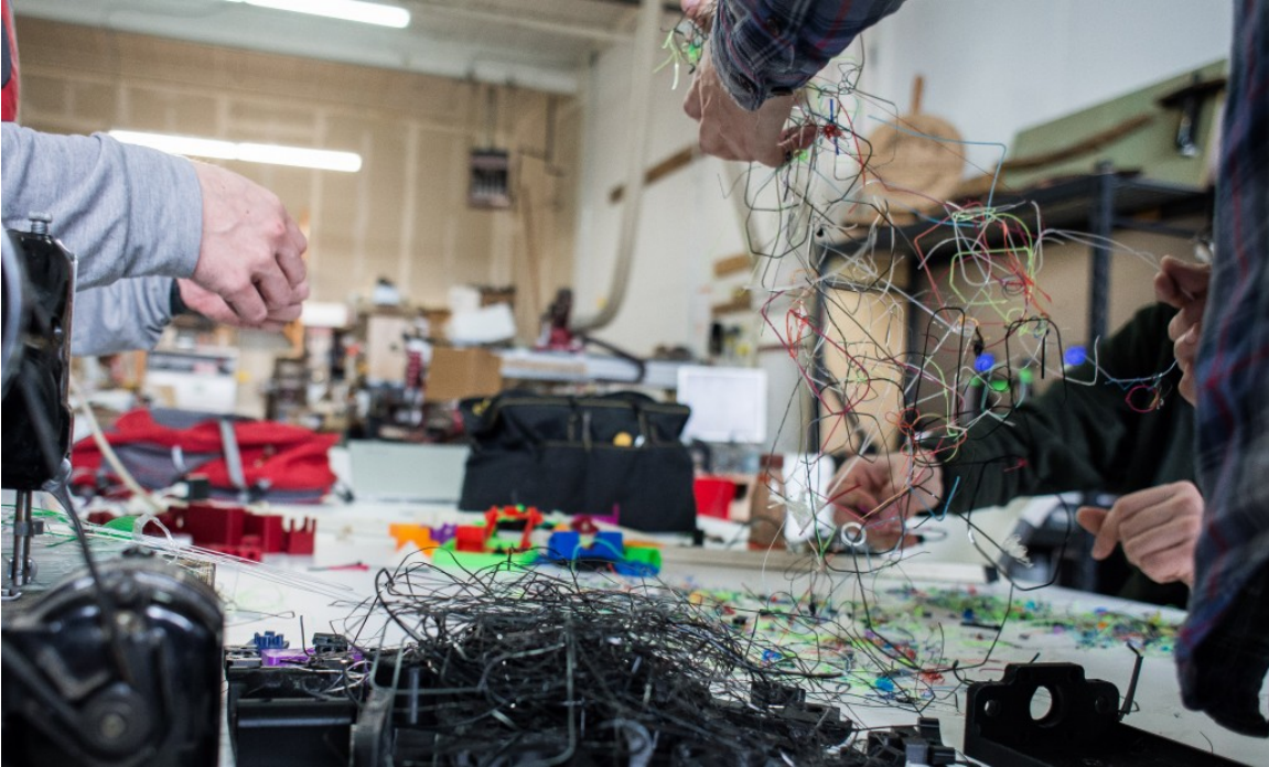
Figure 4. (Literally entangled) 3D printer filament waste being sorted for recycling. Photo by Daniel McNair.
