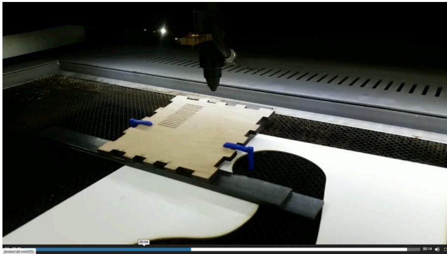
Figure 3. 3D printed clamps (blue) are pictured in this still from a time-lapse video created by Tony Loiseleur and posted on the SMS blog in February 2016.
