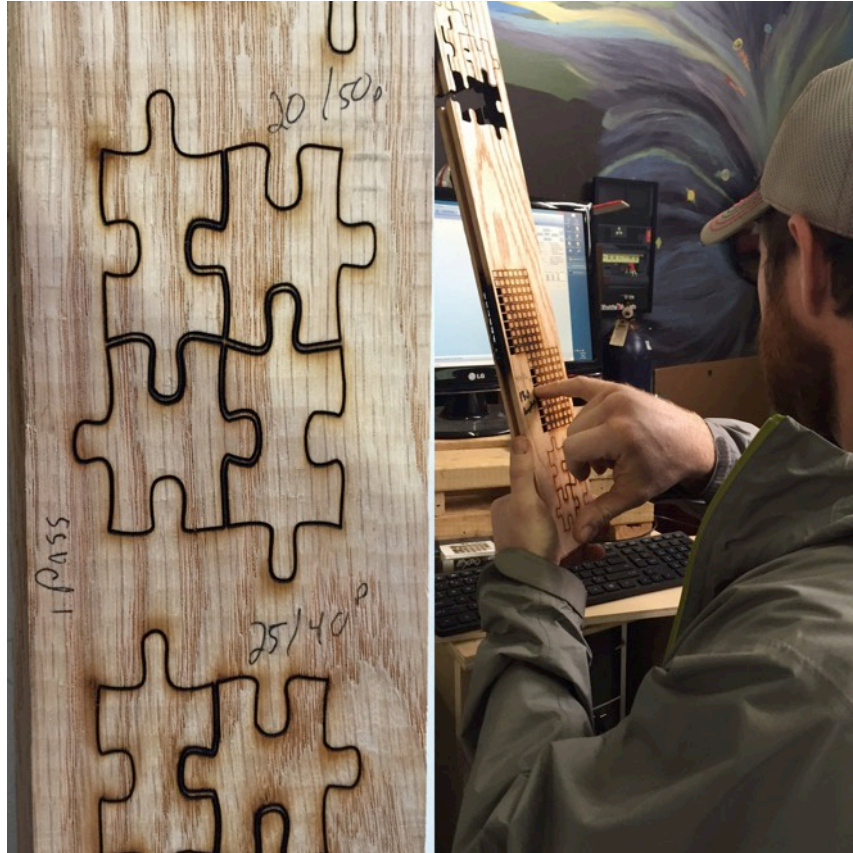
Figure 6. Left: a close up of the flooring piece Eric was experimenting on, with notes on the strength and power settings and number of passes for a series of cuts. Right: Eric consults another section of the practice piece with a small strength/power test grid.
