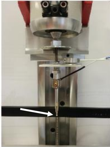
Figure 2.3. Spinal cord contusion injury device. We produced unilateral spinal cord contusion injuries using a modified Ohio State injury device. To stabilize the vertebral column during the spinal injury, we suspended animals with clamps attached to the horizontal black bar. This device produced contusion injuries with a 2 mm wide probe (white arrow) that pressed 0.7 mm deep into the exposed spinal cord for 14 ms.
