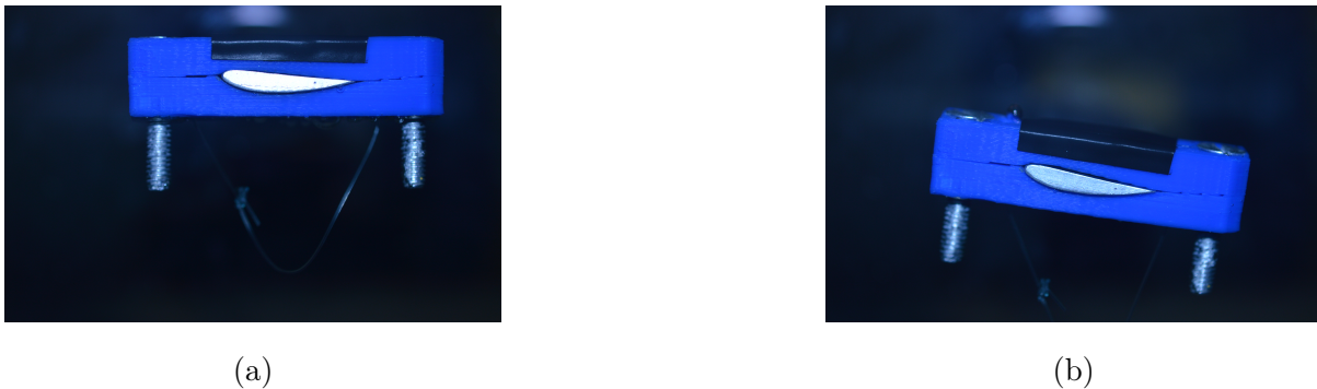
Figure 4.3: For the in-water static test, deflection and twist are determined from photographs taken in the (a) unloaded and (b) loaded states.
