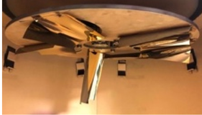
Figure 5.3 PET falls and curls inward after the metal deposition
