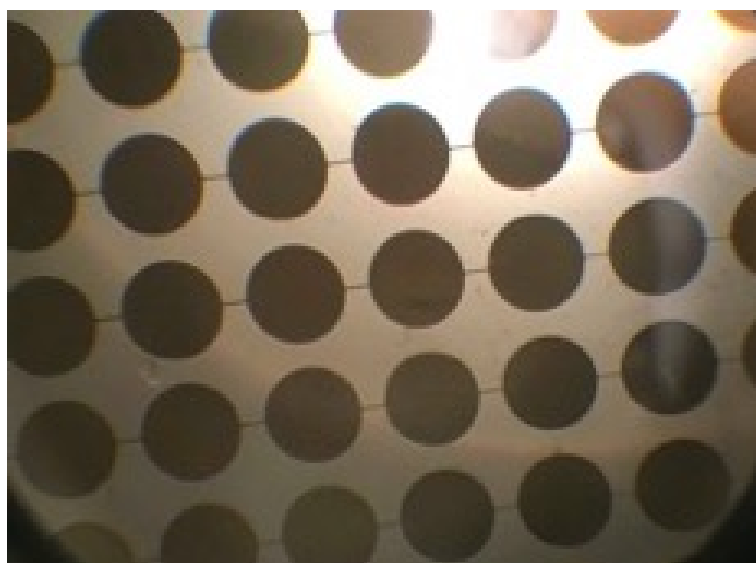
Figure 5.10. The etching result of the sample under the microscope. The connection of electrode arms is carefully checked under the microscope right after the etching.
