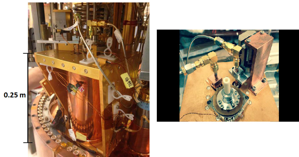
Figure 3.17: ADMX Sidecar is a smaller cavity mounted directly above the main cavity. Sidecar serves as a development test bed and searches for high-mass axions with stronger than DFSZ coupling. The use of piezo-electric motors for tuning will be critical in future ADMX configurations that rely on multiple cavities tuned to the same resonant frequency. Left: Photo of the sidecar cavity mounted to the top of the main cavity. Right: Photo of the piezoelectric motors for tuning sidecar mounted to the top of the sidecar cavity.
