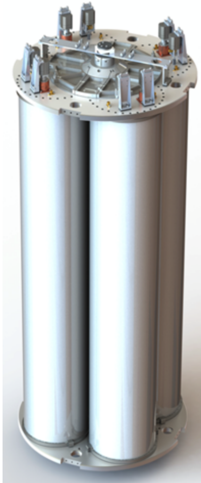
Figure 3.18: A sketch of the ADMX 4 cavity array which will be used to conduct higher-mass axion searches. This will be operational in 2023.
