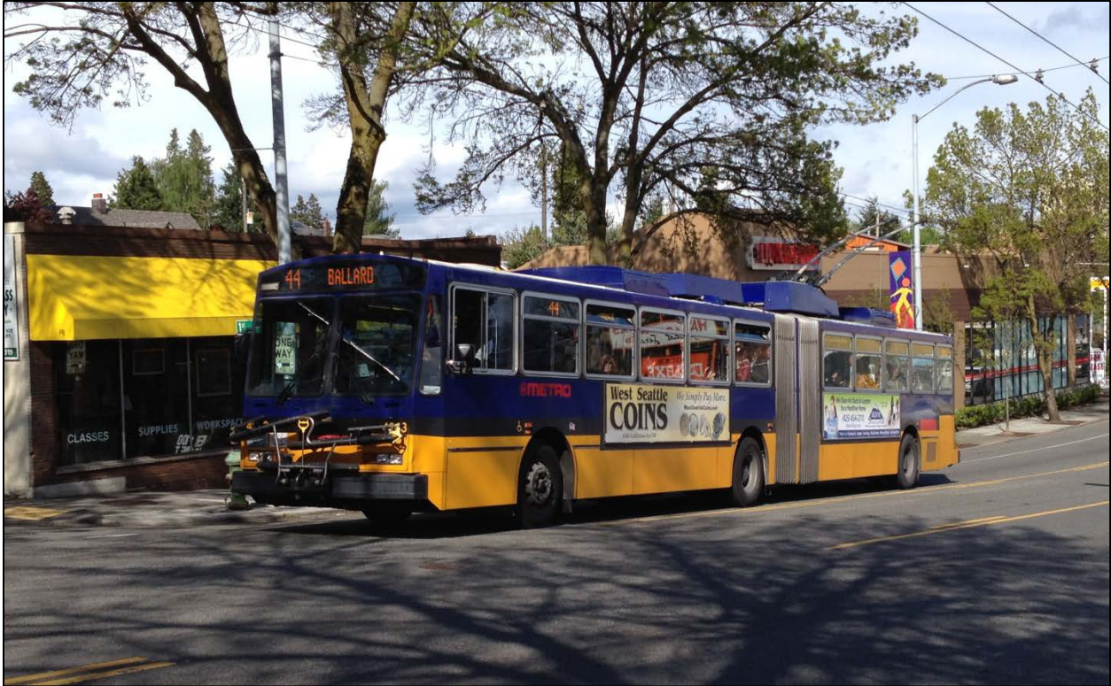
Figure 8 Coaches used on Route 44 have three doors for entry and exit and utilize Seattle’s electrified trolley system
