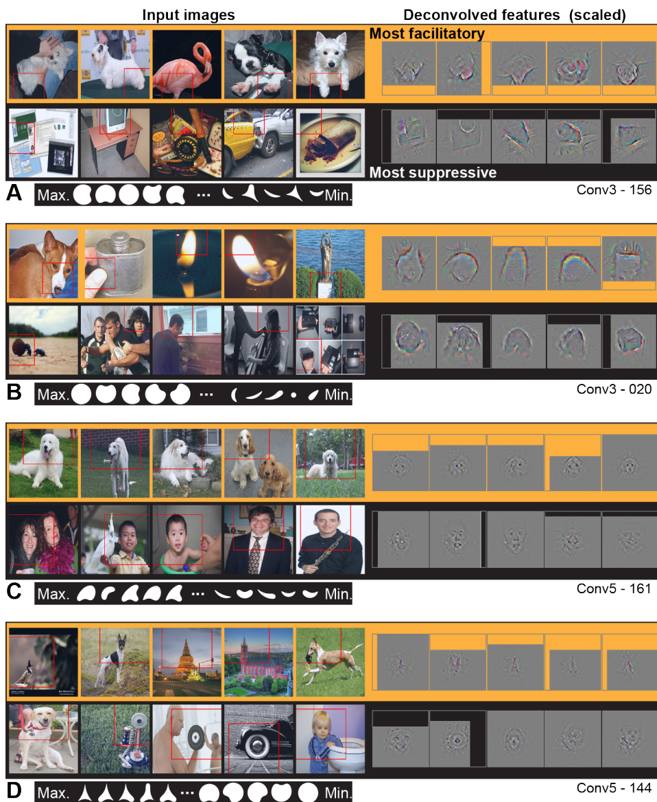
FIGURE 2.12: Visualization of APC-like units in layers Conv3 to Conv5. (A) Visualization for unit Conv3-156, using the same format as Figure 2.11. Deconvolved features are scaled by 1.8 for visibility. (B) Same as (A), for unit Conv3-020. (C) Same for unit Conv5-161, but deconvolved features are scaled by 1.15. (D) Same as (C), but for unit Conv5-144. For APC fit parameters, see Table 1 in main text. The un-redacted input image thumbnails were accessed via the ImageNet database and the original image URLs can be found through this site ( http://image-net.org/about-overview ). These thumbnails may be subject to copyright. They are not available under CC-BY and are exempt from the CC-BY 4.0 license.
