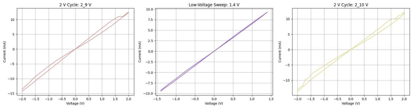
Figure 4.24 ( Left ) First full \pm 2 V sweep showing the baseline switching response. ( Middle ) Narrow \pm 1.4 V sweep producing a linear I–V curve indicative of ohmic conduction with no resistive switching. ( Right ) Second full \pm 2 V sweep after low-voltage cycling.
