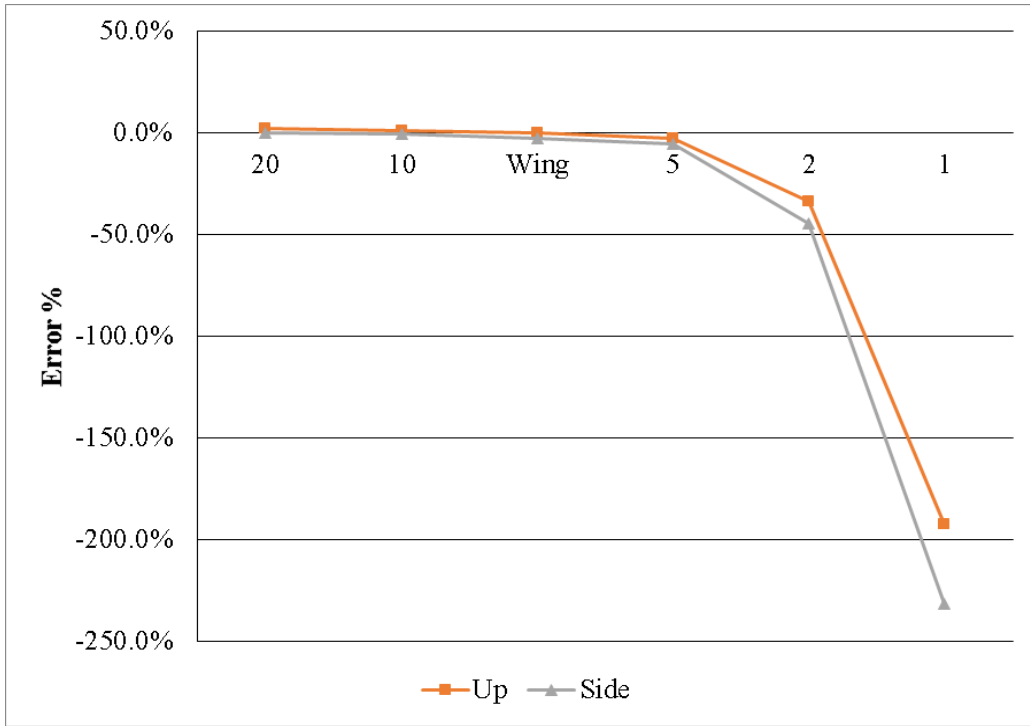
Figure 4.15: Titanium Box Beam, Error Percentage vs. Length:Width Ratio
