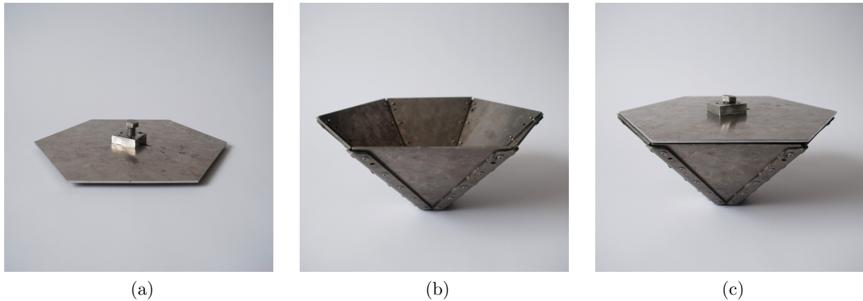
Figure 3.1: Three experimental test articles with varying topology: (a) flat plate, (b) open conic, and (c) enclosed conic.
