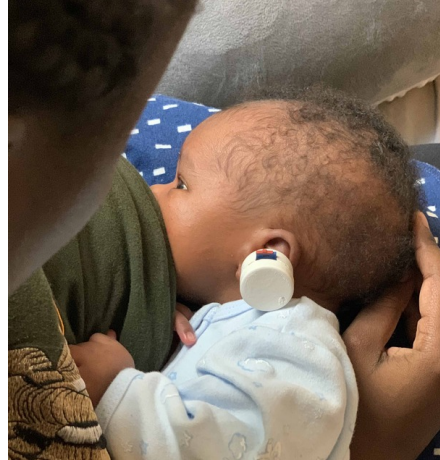
Figure 4.1: OAEbuds in use with an infant. Our low-cost wireless earbud can perform hearing screening by detecting otoacoustic emissions (OAE) from the cochlea.
