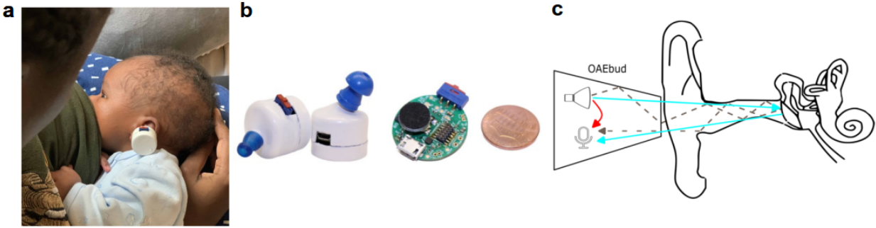
Figure 1.3: Wireless earbuds for low-cost hearing screening. a , OAEbuds in use with an infant. Our low-cost wireless earbud can perform hearing screening by detecting OAEs from the cochlea. b , Wireless OAEbuds hardware. c , Our algorithms combine frequency modulated chirps with wideband pulses emitted from a low-cost speaker to reliably separate OAEs from in-ear reflections and echoes.
