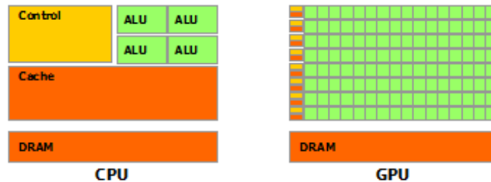
Figure 2.2: Architecture difference between CPU and GPU (adapted from CUDA Programming Guide, NVIDIA Corp).
