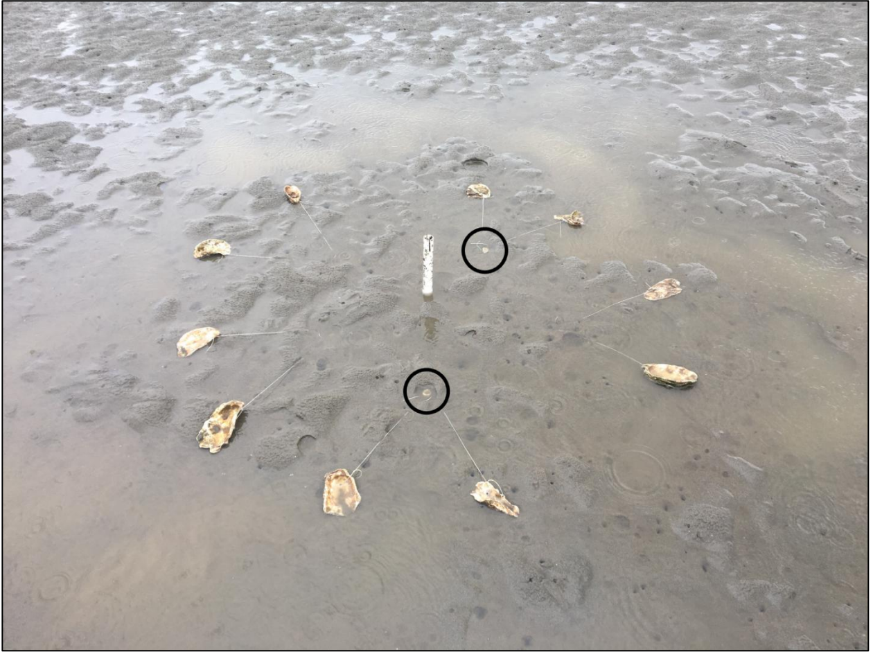
Figure S3. Seeded cultch deployed at a site with high burrowing shrimp density, also showing the water content at low tide. Each PVC pipe (shown within black circles) has two pieces of seeded cultch for a total of 10 pieces per site.
