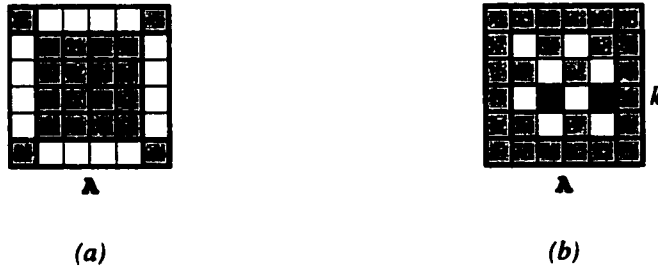
Figure 2.10: Region Inheritance Examples. In both diagrams, white is used to represent 0, black to represent 1, and grey to indicate values that are untouched. (a) The result of the assignments using double-quote references in Listing 2.10. (b) The result of the statements in Listing 2.11 using the same checkerboard mask as Figure 2.9.
