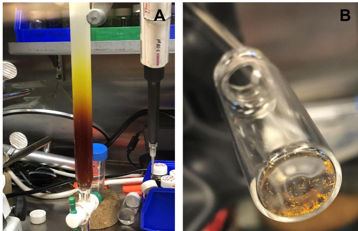
Figure 3.3.2. A) Direct purification of an InAs nanocluster reaction by size-exclusion chromatography. The yellow band is the \text{In}_{26}\text{As}_{18} cluster and the dark red band is quantum dot impurity. B) Photograph of the isolated single crystals grown from an ether against pentane vapor diffusion.
