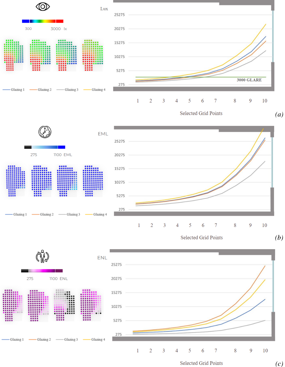
Figure 4.8 Horizontal Grid Simulation and Illuminance Curve of Selected Grids to Compare the Impact of Four Glazing Types for (a) Photopic, (b) Melanopic, and (c) Neuroptic Light Simulation Results
