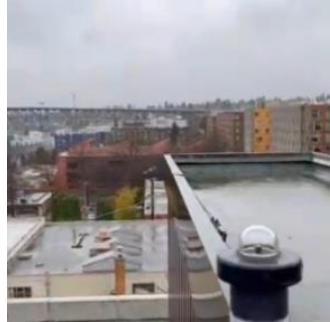
Figure 3.5. A Spectrometer on the Roof of a Gould Hall is Measuring the Spectrum of Daylight in Seattle.
