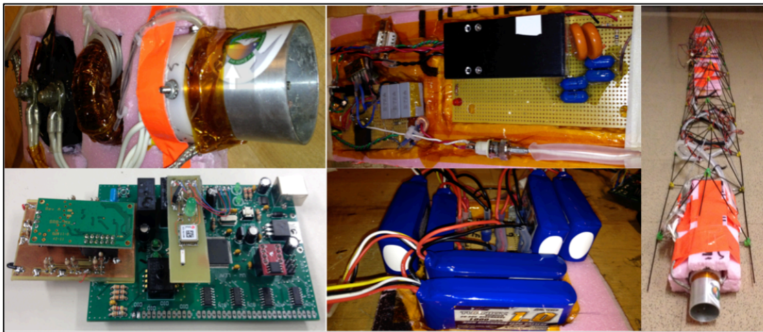
Figure 7.16. The PPT electrodes and main discharge energy storage (top left), igniter and main discharge circuitry (top center), ATMEGA1280 microprocessor (bottom left), LiPoly battery pack (bottom center), and thruster housed within a single 8ft carbon fiber truss structure (right).
