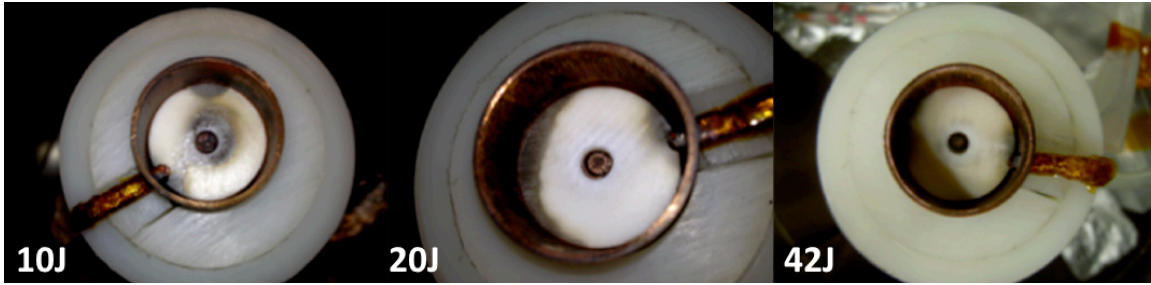
Figure 4.4. PPT surface charring after 150 shots at a base pressure of 1 \mu Torr for discharge energies of 10, 20, and 42J (left to right).
