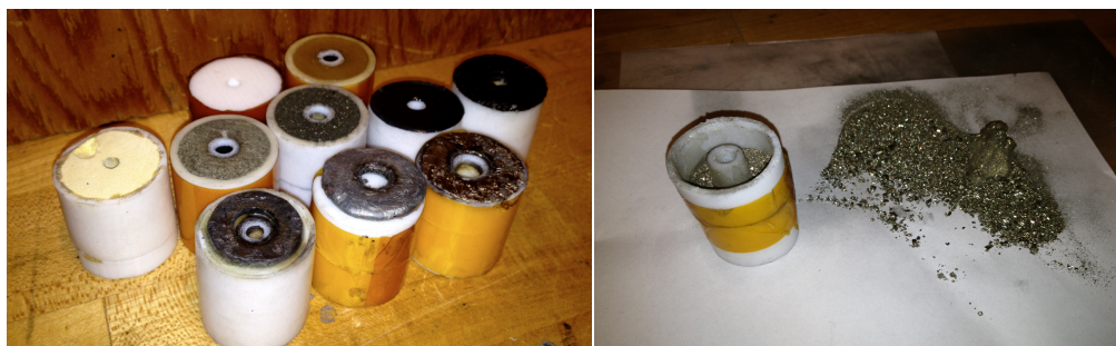
Figure 5.11. The ten propellants tested, Teflon and epoxy (left to right, top row), sulfur, olivine, chalcopyrite, bismuth sulfide, and volcanic ash (middle), lead, gallium, and bismuth (bottom). A Teflon insulator and chalcopyrite grains (right).
