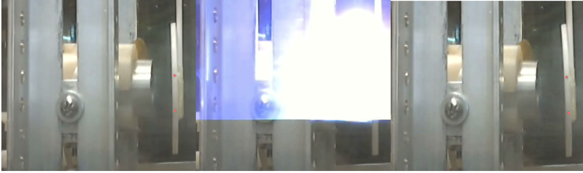
Figure 3.9. The recorded video of the pendulum before firing, at firing, and at the peak deflection angle which occurred 4-6 frames after the discharge depending on the impulse (left to right).
