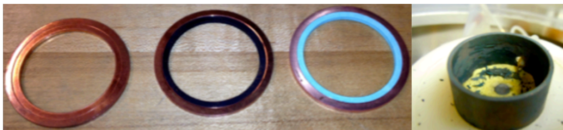
Figure 5.10. Copper gaskets used while testing with sulfur for durations of (left to right) one week, one month, and one year and a sulfur propellant thruster with copper electrodes after 100 43J discharges (far right).
