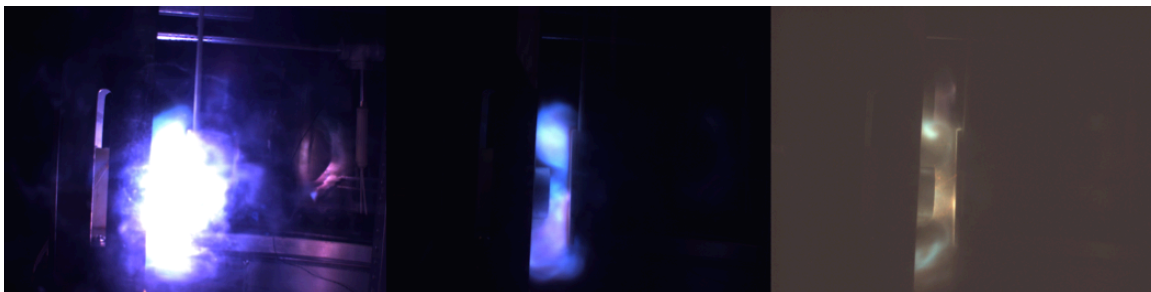
Figure 6.2. High speed imagery taken with the camera set to a high exposure at discharge times of 0-100 \mu\text{s} , 100 \mu\text{s} – 5ms, 500 \mu\text{s} – 5.5ms (left to right) relative to the igniter discharge for a 32J main discharge.
