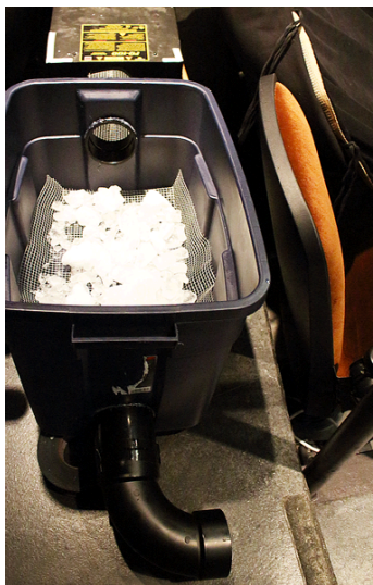
Figure 22: Fogger and fog chiller used in the Horizon is an Imaginary Line
