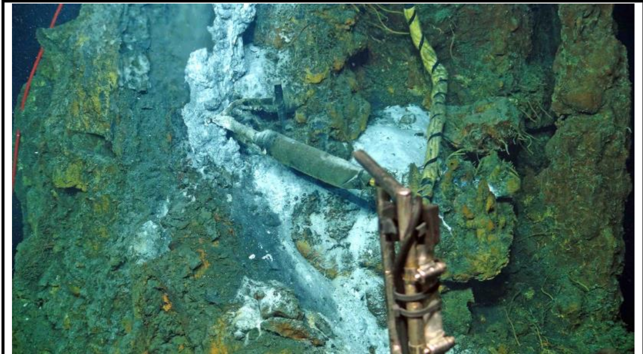
Figure 4. The temperature and resistivity probe embedded in the Escargot hydrothermal chimney (in the International District Hydrothermal Vent Field) at a depth of 1520 m. The probe was developed for the Regional Cabled Array by Dr. Marv Lilley of the University of Washington. It was installed in September 2014. Image retrieved from: https://interactiveoceans.washington.edu/instruments/resistivity-temperature-probe/
