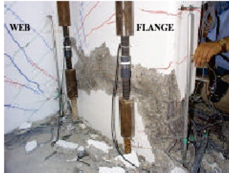
Figure 3.12: Failure of one flange for the specimen IleXY loaded bi-directionally [29]
