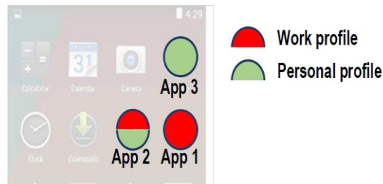
Figure 3.2. The owner of “work” approves App1 and App2, but does not trust App3 approved in “personal”
