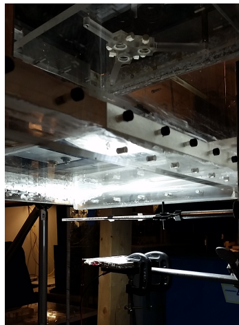
Figure 3.20: Illumination setup for the calibration configuration
