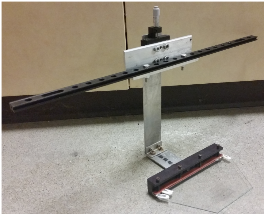
Figure 3.14: The calibration rig used in this study consisted of a single-axis translation stage and calibration target plate.
