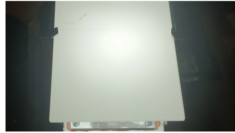
(b) Diffusor plate used to smooth illumination distribution
