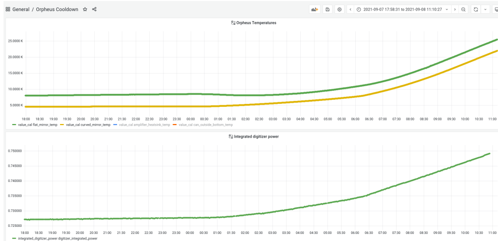
Figure 6.5: Plotted integrated digitizer power as the cavity is warming up. For reasons outlined in the text, this measurement is difficult to interpret as a Y-factor measurement to obtain the receiver noise temperature. But the digitized power rises more-or-less linearly with the cavity temperature. This suggests a healthy, low-noise receiver chain.
