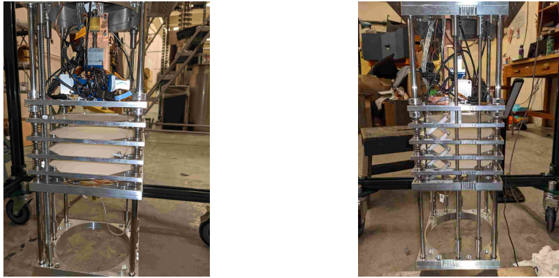
Figure 4.4: Orpheus cavity attached to the cryogenic insert.
