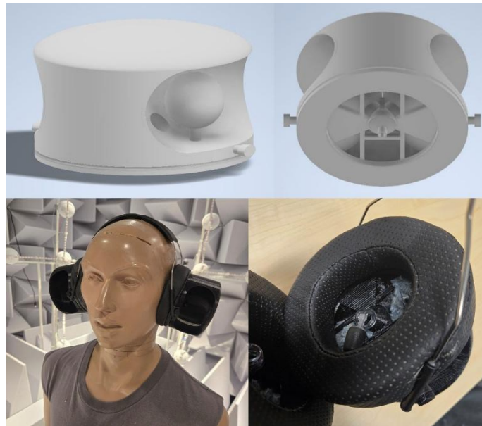
Figure 2. 3D rendering of the designed earmuff (top) with symmetrical cavities. A Helmholtz resonator tuned to 2 kHz can be seen in the rear cavity. Tubing is used to couple the earmuff to a Comply® Foam ear tip (bottom right). The earmuff is attached to a headband and worn by a KEMAR manikin for acoustic testing (bottom left).
