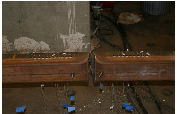
Brace Fracture: 2.08" T1 cycle
