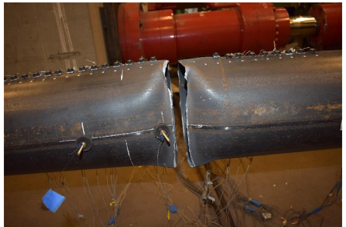
Brace Fracture: 2.25" T2 cycle
