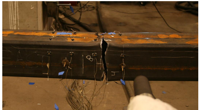
Brace tear >50%: 1.25" T1
