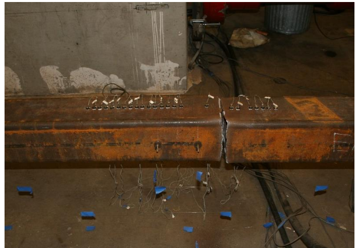
Brace Fracture: 1.62" T1 cycle
