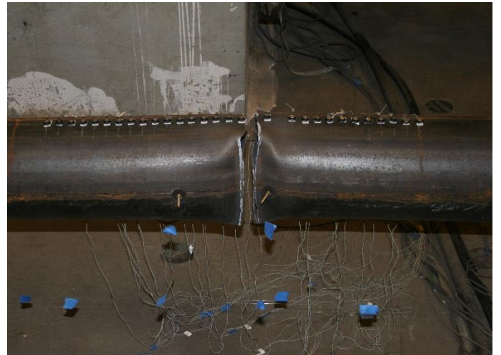
Brace Fracture: 2.25" T2 cycle
