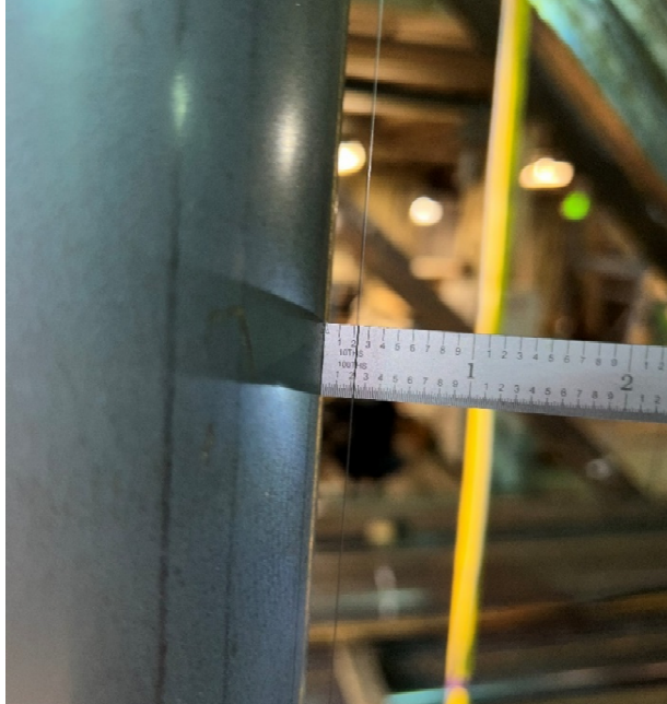
Figure 3.17 Measurement of Imperfection at Midspan
