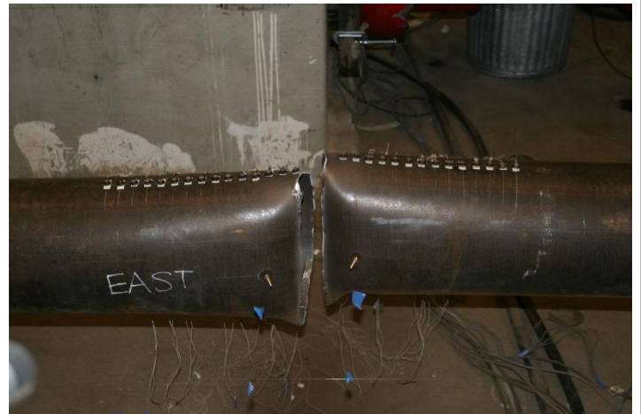
Brace Fracture: 2.25" T1 cycle
