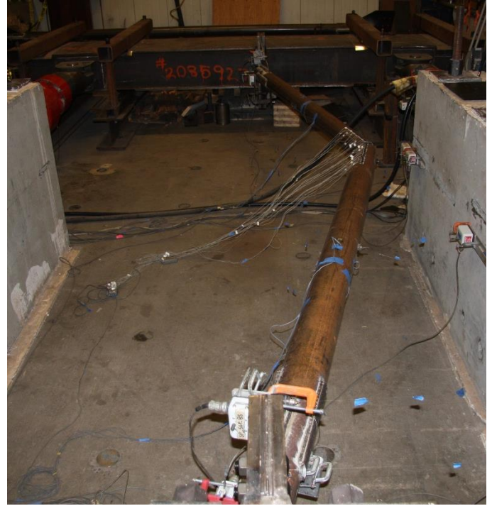
Buckling After Partial Tear: 3.00" C2 cycle
