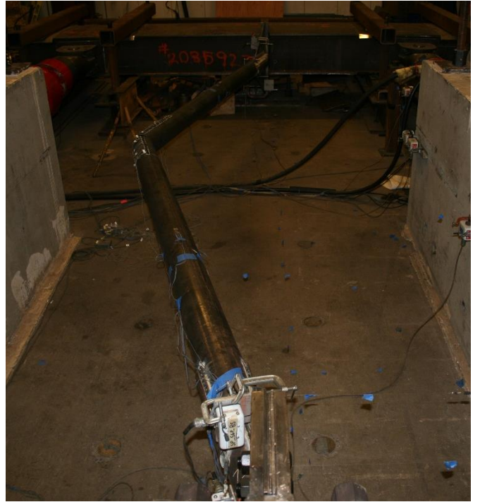
Buckling After Partial Tear: 3.93" C2 cycle
