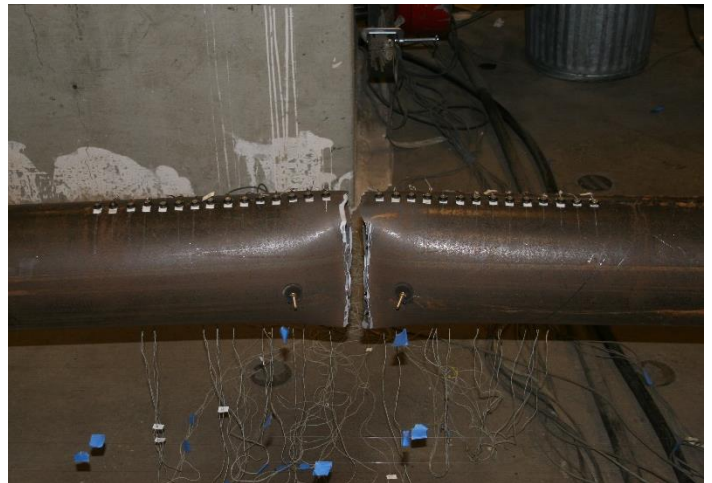
Brace Fracture: 3.25" T1 cycle
