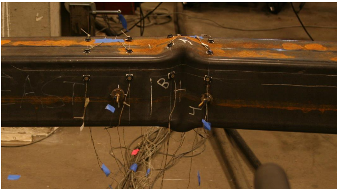
Major Cupping ~3.5" north of center: 0.75" C2
