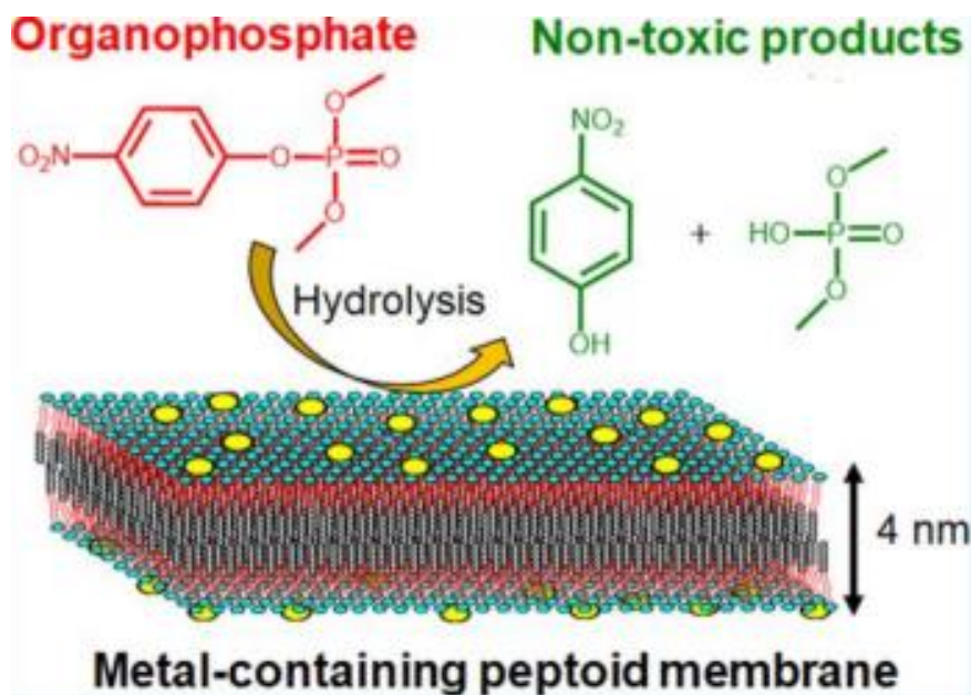
Figure 1-12 Metal-containing peptoid membrane for OP degradation
