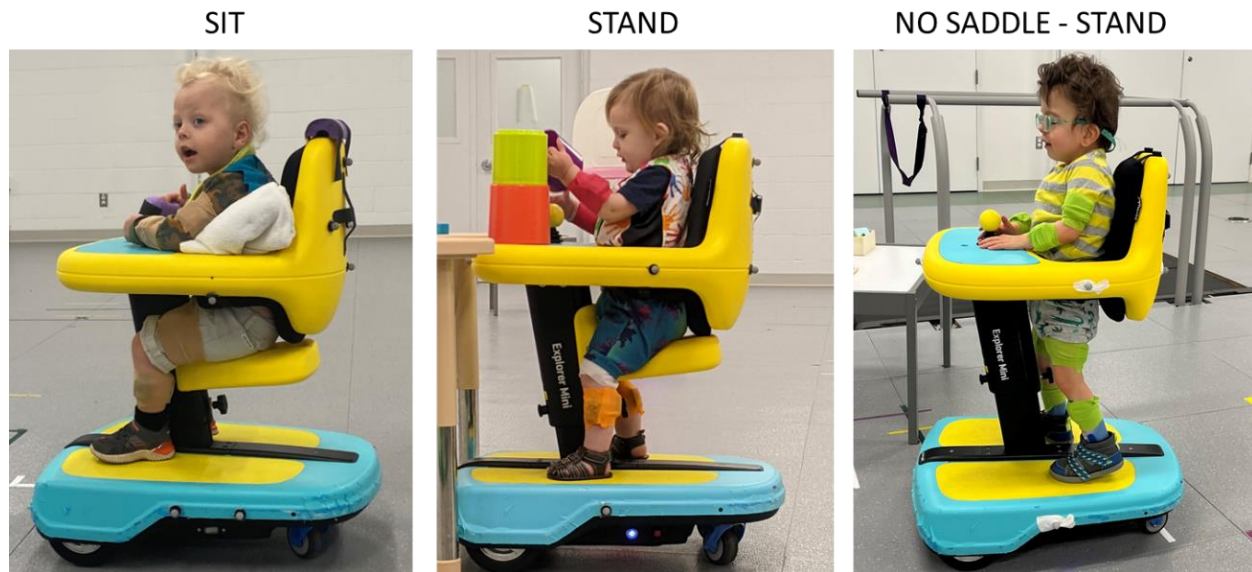
Figure 6.1 Comparison of posture configurations. From left to right: SIT, seated with saddle and knees \sim 90^\circ , STAND, supported standing with saddle and knees near to 180^\circ , NO SADDLE - STAND, unsupported standing with no saddle in place.
