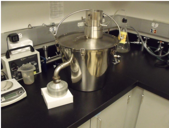
Figure 2.2. Custom-built Soil Aerosolization Chamber (SAC) for generation and collection of soil aerosols prior to primary plating.
