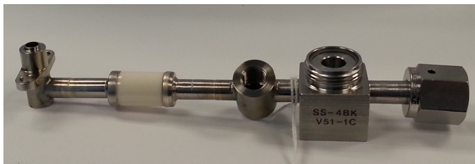
Figure 3.9: Valve base assembly. The opening at far left holds a Viton o-ring on the shoulder and secures to the injector with two screws. The ceramic insulator is to its right, followed by a socket for a PCB Piezotronics S112A21 pressure sensor. To the right of that is a Swagelok valve base with the downstream VCR fitting cut off.
