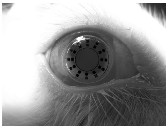
Figure 23. Image of a contact lens with a 2 x 12 solar cell array placed on a live rabbit eye.
